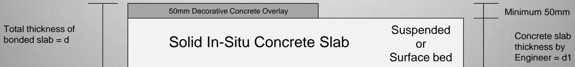
maximum length of panel size = 30 times the total thickness (  $d$  )
