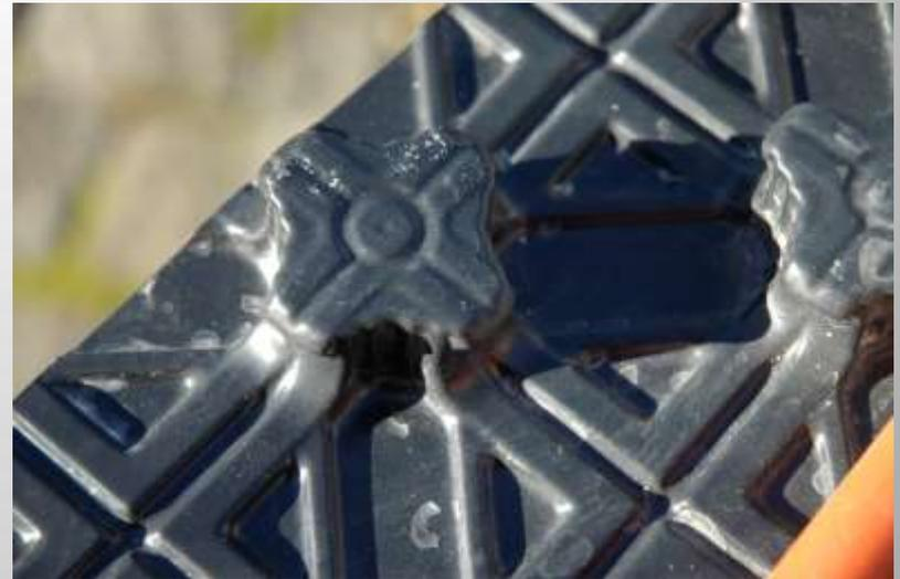
Typical Mushroom that hold the pipes and bond to the concrete
